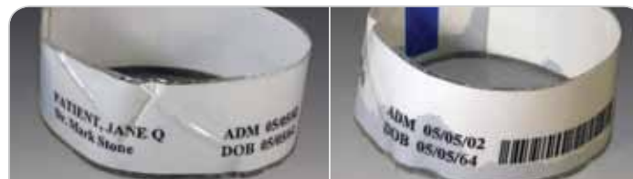
Using a laminate overlay wristband can cause wrinkles and folds (top left). Also, water and chemicals can become trapped underneath, corrupting critical data (top right). These defects can obstruct scanning.
